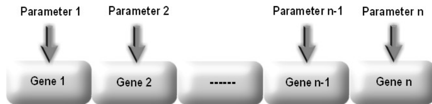
Figure 2. Encoding of the solution parameters as genes of a chromosome consisting of 36 bit.
