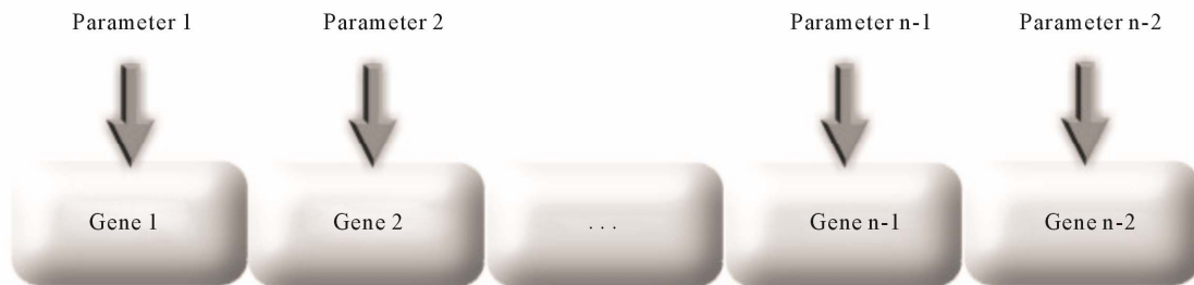
Figure 7. Encoding of the solution parameters as genes of a chromosome.
