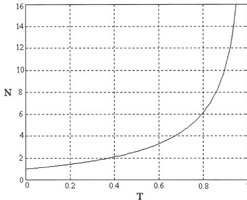
Fig. 9. Magnifying factor  $N$  as a function of the trapping percentage  $T$  of the beam.
