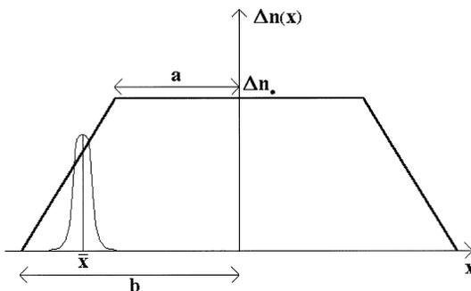
Fig. 1. Section of the ideal trapezoidal refractive index profile waveguide.
