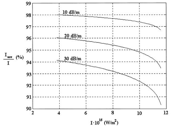
Fig. 8. Ratio between the output intensity with absorption and the output intensity without absorption (percentage) versus input intensity for different values of the absorption coefficient of the medium.
