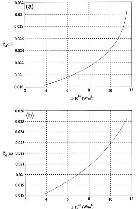
Fig. 7. (a) Detach distance as a function of the input intensity without absorption. (b) Detach distance as a function of the input intensity for an absorption coefficient equal to 30 dB/m.
