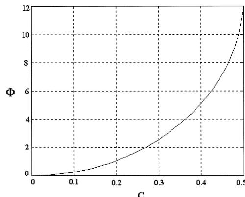
Fig. 3. Detach angle  $\Phi$  in degrees, equal to  $\arctan(v_D)$ , versus  $C$  for  $v_G = 0.224$  (waveguide inclination:  $12.6^\circ$ ),  $\Delta n_0 = 0.05$ . The detach value is  $C_D = 0.5$
