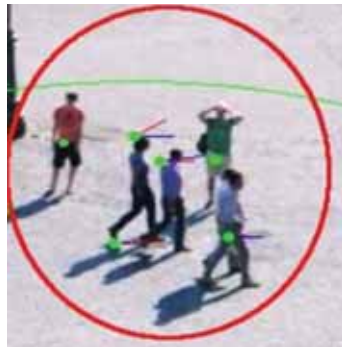
Figure 3: Pedestrian state prediction module output where the darker vector is the measured speed and the whiter vector is the predicted one.
